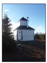
(Big) Swede Lookout Project - Kootenai National Forest — This project was divided into two parts. The first part consisted of volunteers glazing 52 windows, replacing catwalk posts, railing, and landing posts. The second project consisted of scraping, sanding and painting the lookout. In 2019 a new roof was put on and additional stabilizing of the roof in 2020.
